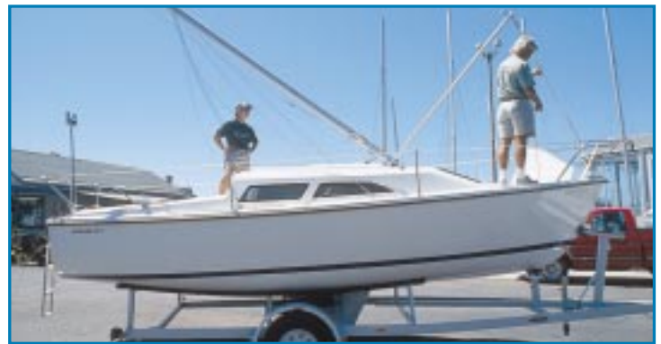
The mast raising system makes pre-launch preparation fast and easy.
